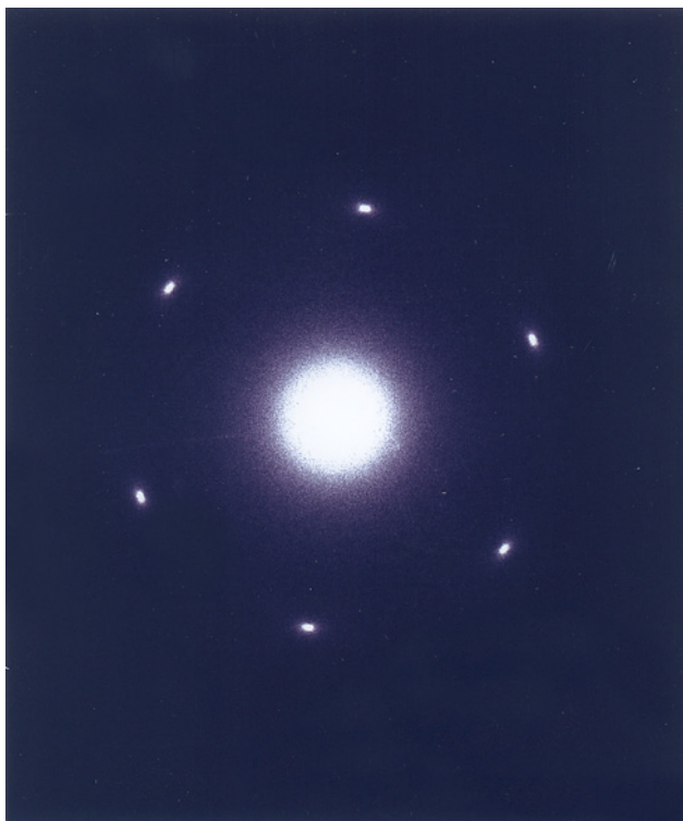
FIGURE 4 Electron diffraction pattern of a 6-layer 4O.8 film at 47.0°C. (See COLOR PLATE III)
